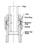
**6.** The maximum sealing pressure for these fittings is 150 PSI.
